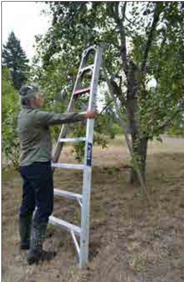
Figure 6.2: (right) Place body weight on the bottom rung to dig the ladder’s feet into the soil.
