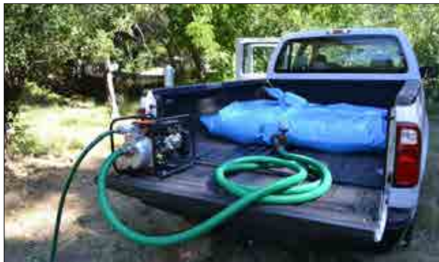
Figure 6.41: 250 gallon collapsible water bag, pump and suction hose on Ford F250.
