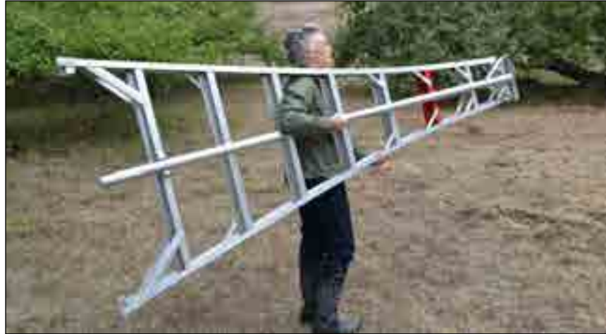
Figure 6.5: The proper way to carry an orchard ladder is over the shoulder.
