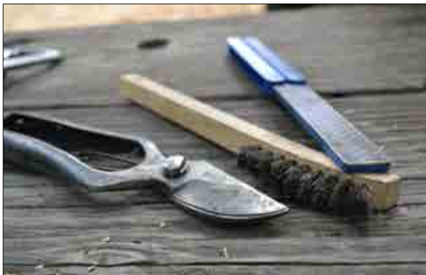
Figure 6.10: Bypass pruners with wire brush for cleaning pruners and file for sharpening pruner blades.
