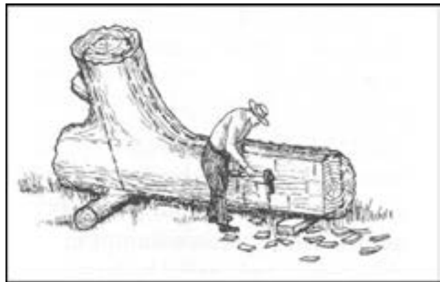
Figure 3-11: Hewing a knee from a piece of 'compass timber'
